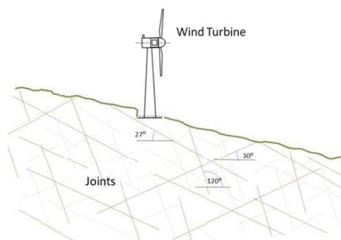
Figure 4. Cross section of the rock mass where the wind turbine is going to be installed.
