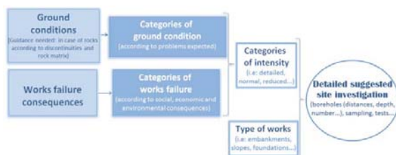
Figure 1. Process to define categories of intensity of site exploration.
