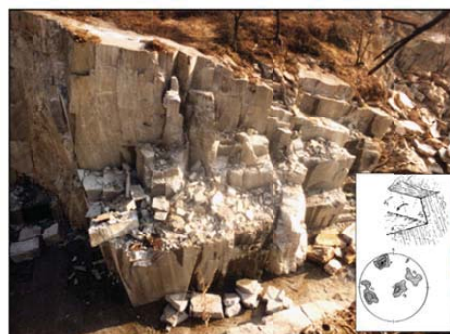
Figure 11. A slope in a quarry in the Alps showing a typical block toppling failure mechanisms and equal area projection of the discontinuity poles of the rock mass (right hand side).
